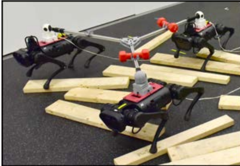
Figure 4.1: Snapshot showing the locomotion of three holonomically constrained A1 robots on wooden blocks.
