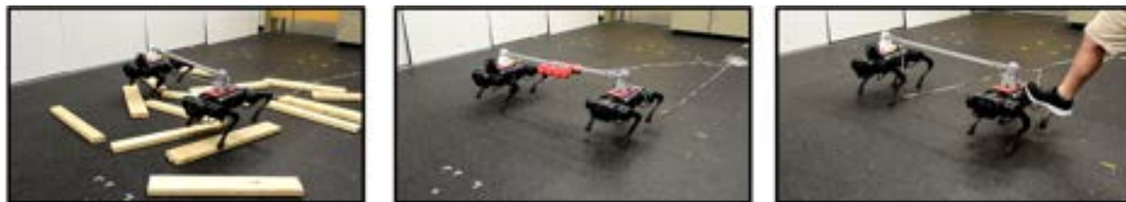
Figure 5.7: From left to right, this figure shows snapshots of locomotion subject to unstructured terrain, a 9 kg payload (75% of the mass of one agent), and extensive pushes.
