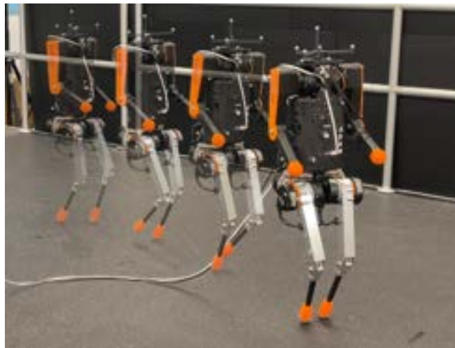
Fig. 1: Snapshots of ADAM tracking the nominal HZD gaits with a stabilizing HLIP controller.
